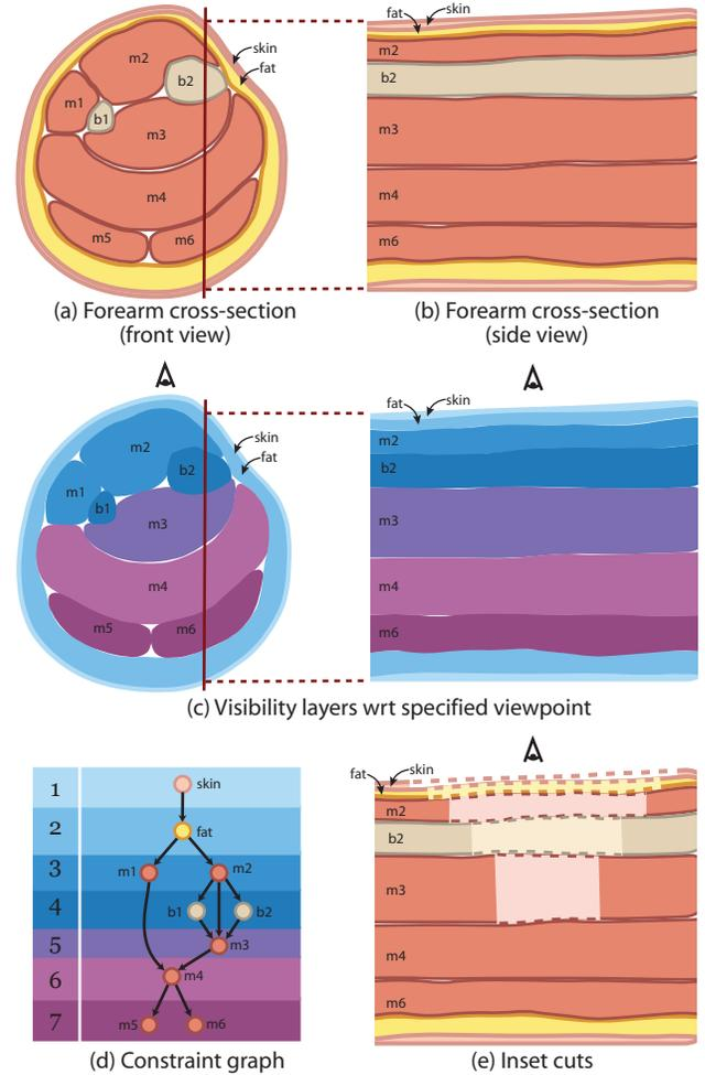
**Figure 12:** Computing constraint graph. (a)-(b) Forearm cross-section viewed from front and side. (c) Structures sorted into visibility layers based on depth complexity from specified viewpoint. (d) Directed edges from occluders to occluded parts are added to graph. Edges flow only from lower to higher layers. (e) Nodes are sorted in topological order to produce a set of inset cuts.
