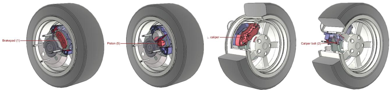
**Figure 16:** Automatically generated cutaway views of disk brake model. We generated an illustration for each of the 27 parts in the model. Here, we show four representative images that use both saved viewpoints. The image on the right shows an artifact; the cuts that expose the target part also leave it disconnected from the surrounding parts. Out of the 27 illustrations, one other exhibited a similar artifact.
