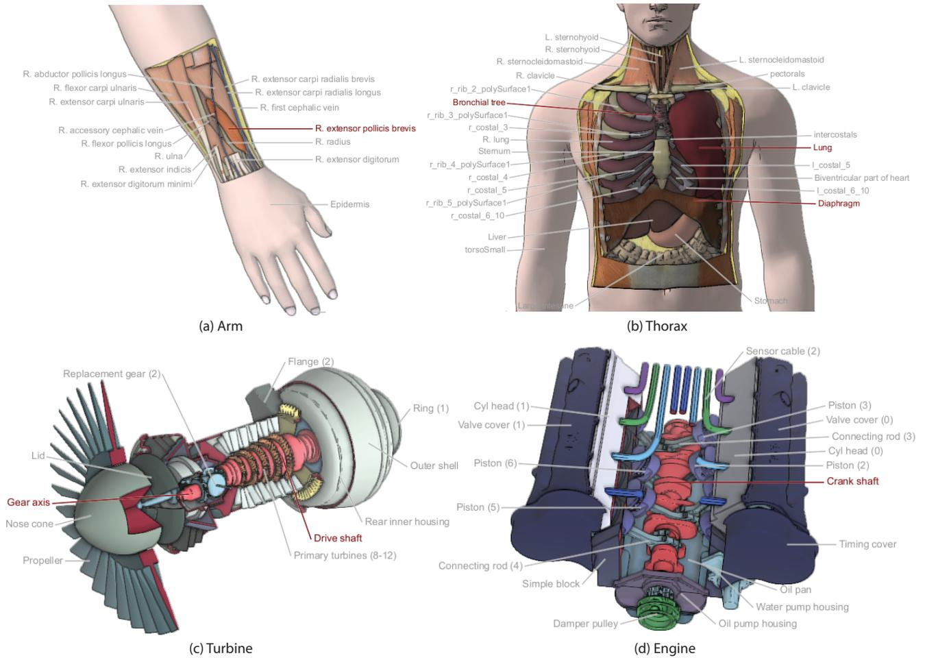
**Figure 15:** Illustrations generated using our automatic cutaway generation interface. A combination of window and transverse tube cuts removes the layers of skin, muscle and bone that occlude the target muscle in (a) and the internal organs of the thorax in (b). Extruded angle tube cuts expose target parts within the turbine (c). Axis-aligned and transverse tube cuts reveal the engine’s crank shaft (d). In (c) and (d), cut surfaces are highlighted in red.
