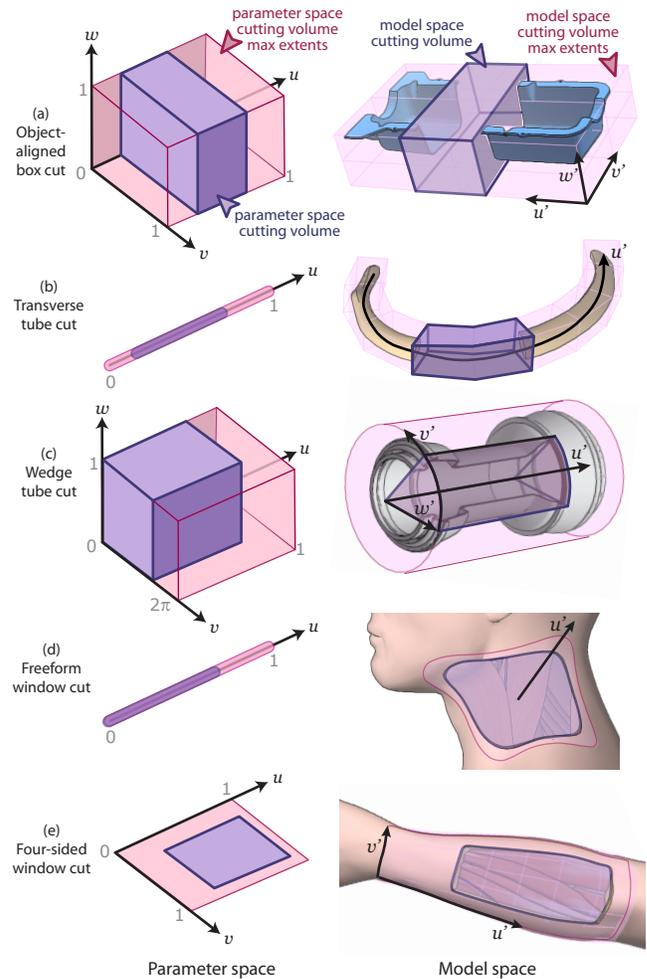
**Figure 8: Cutting volumes.** In our system, a cut is represented as a cutting volume that is defined in a one-, two-, or three-dimensional parameter space (left column) and then mapped to the model’s local coordinate system (right column). For each type of cut, the cutting volume (purple) and its maximum extents (pink) are shown in both parameter and model space. The model space mappings  $u', v', w'$  of the parametric dimensions  $u, v, w$  are also illustrated on the right.
